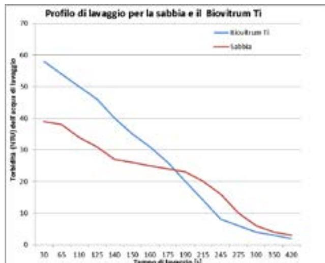
The curve shows the water consumption while backwashing a filter filled with sand compared to that of a filter filled with Biovitrum Ti.
